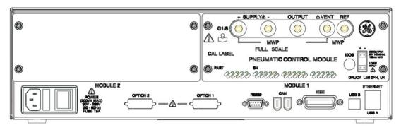
Figure 2-2, Pressure module rear view
