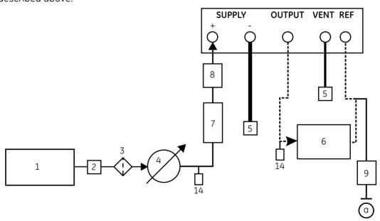
Figure 2-3, Pneumatic Connections without vacuum supply
