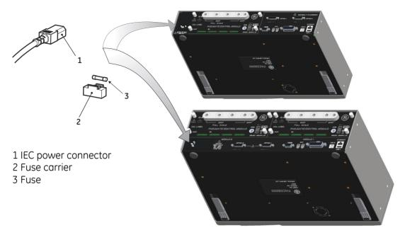
**Figure 2-7 Electrical Connections**
