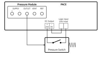
**Example Switch Test Connections**
