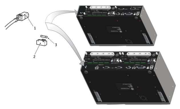
1 - IEC connector 2 - Fuse carrier 3 - Fuse
