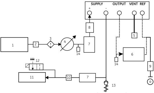
Figure 2-4, Pneumatic Connections with vacuum supply
