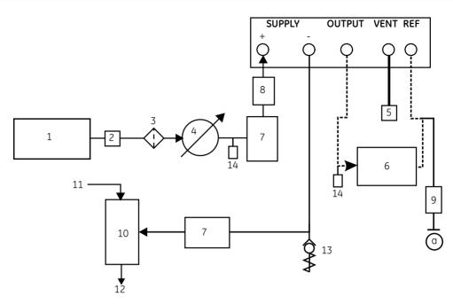
Figure 2-5, Pneumatic Connections with negative gauge pressure generator
